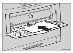
Load adhesive labels into the tray with the print side face down.
